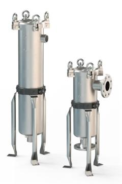
The medium enters the housing by the sideward inlet. All solid matter contamination remains in the filter bag and the cleaned filtrate leaves the housing by the outlet in the bottom.
